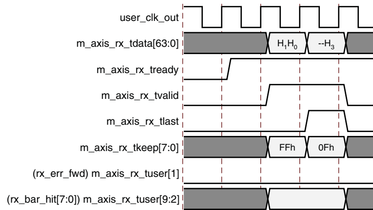
Figure 3-15: TLP 3-DW Header without Payload
